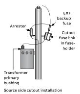
Arreste Cutout EXT use link backup in fusefuse holder 00 Transformer primary bushing
