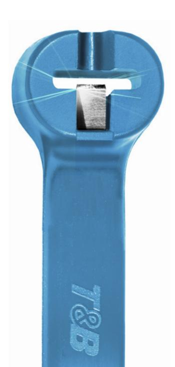
Only Ty-Rap has The Grip of Steel® locking device made of 316 stainless steel, for superior strength in even the harshest environments. The smooth, rounded strap ensures even pressure across the tie and around the circumference of the bundle. Ribs and stipples hold tight during vibration, and the solid body is stress free to prolong the life of the cable tie.
