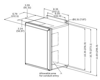
60-200 kA polycarbonate enclosure with termination lugs
