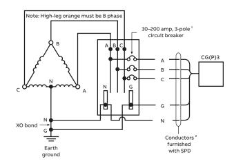
Figure 5: 3-phase high-leg delta, 4-wire
