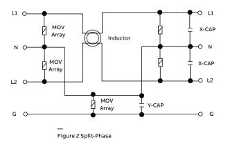
Match the corresponding L1 & L2 terminal lugs for the input & output phase wires when connecting a split-phase configuration.
