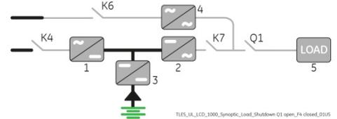
**3. Disconnect the Battery from the UPS by opening the “Battery Cabinet Breaker” (Pos. O).**
