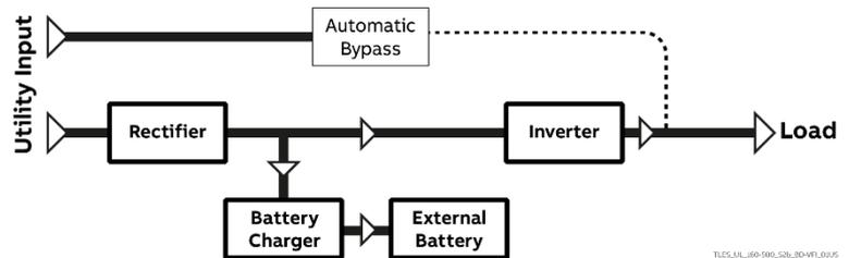
Fig. 4.2.1-1 Block diagram normal operation mode
