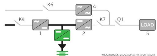
**3. Disconnect the Battery from the UPS by opening the “Battery Cabinet Breaker” (Pos. O).**
