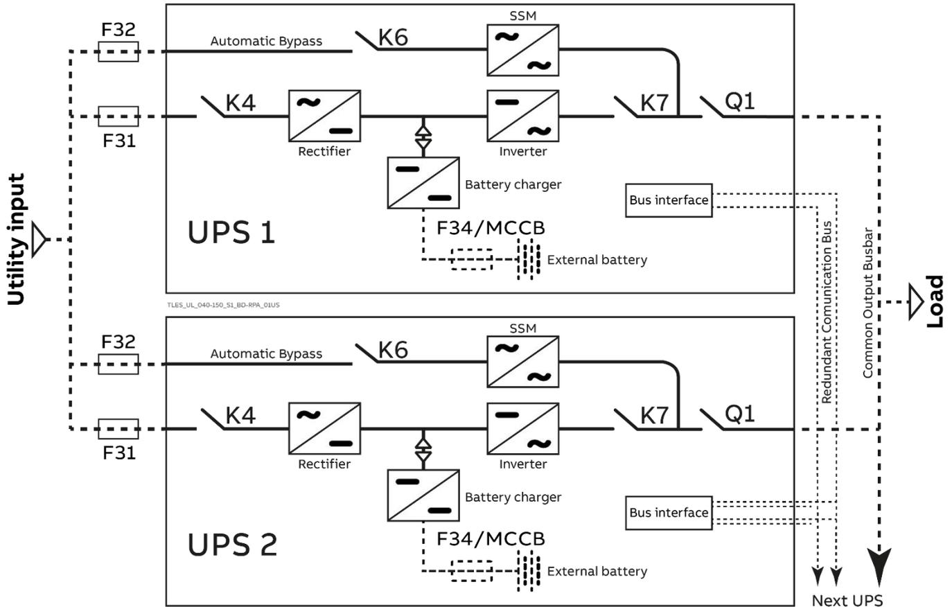
Fig. 4.3.1-1 Block diagram RPA Parallel System operation
