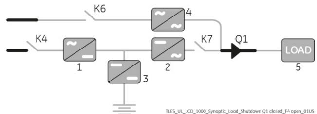
**1. Restore the command “System shutdown” of the RPA Parallel System.**
