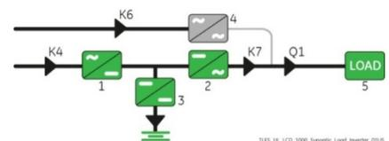
The Synoptic Diagram must display the status “Load supplied by Inverter”.
