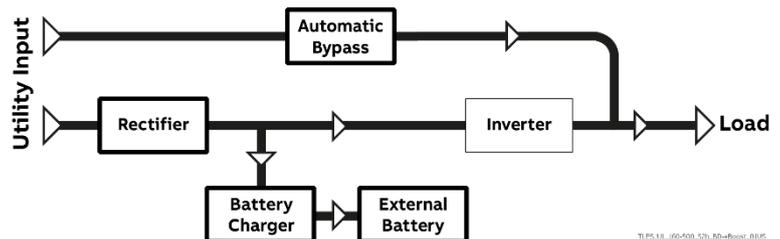
Fig. 4.2.2-1 Block diagram “SEM - Super Eco Mode” Operation Mode
