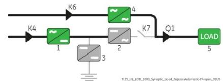
The Synoptic Diagram must display the status “Load supplied by Automatic Bypass”.
