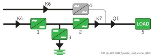
**1. Disconnect the Inverter performing the “Inverter OFF” command on the Unit to separate.**
