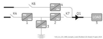
View of the Synoptic Diagram after performed the command “EPO - Emergency Power Off” with Load not supplied.
