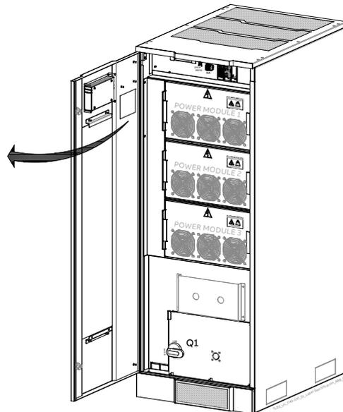
The requested data permitting to identify your UPS are marked on the **identification label** fixed on the front of the cabinet, behind the lower front door.
