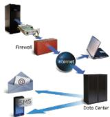
iUPSGuard is a remote monitoring solution for UPS, providing status monitoring and alarm notification that supports all ABB UPS product lines, anytime, anywhere.
