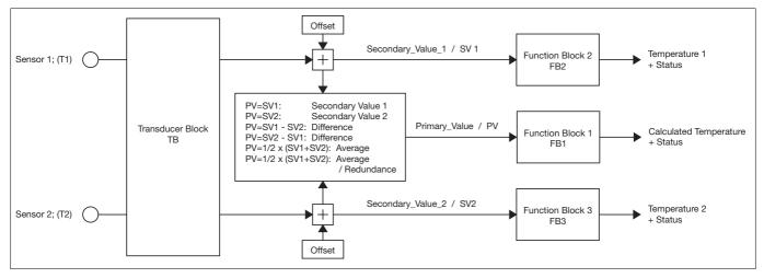
Fig. 2-3 Structure of the temperature transducer TF12/TF212
