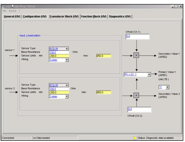
Fig. 2-6 Transducer block (UV)
