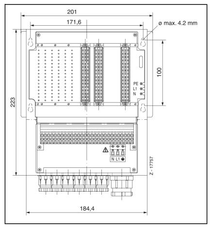
Fig. 16-5 Dimensional drawing of field case (dim. in mm
