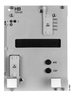
Fig. 16-1 19" plug-in card, front view
