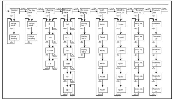
Fig. 20-1 Display and operation with the keys "MOD" and "STEP"
