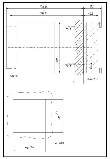
Fig. 16-7 Dimensional drawing of control panel case (dim. in mm)
