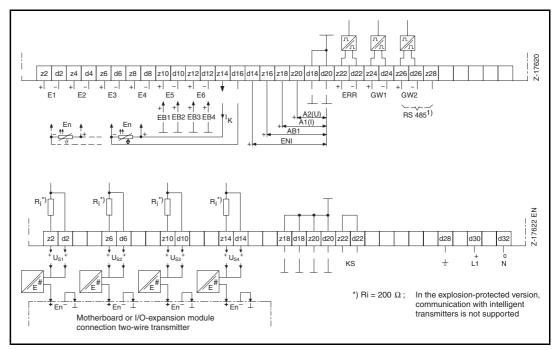
Fig. 19-1 Connection diagram of 19" plug-in card - motherboard (above) and mains card (below)
