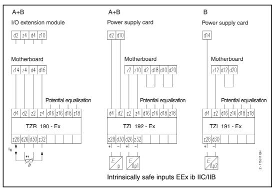
Fig. 19-3 Connection diagram of 19" plug-in card with intrinsically safe inputs via safety barriers for A 1 x Pt 100 direct, 2 x mA B 1 x Pt 100 direct, 3 x mA (see "Expert Commentary" No. 95-04-205-Ex)
