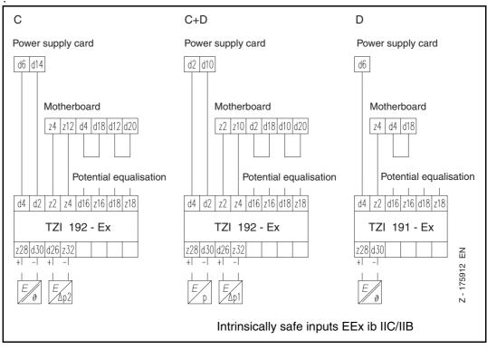
Fig. 19-4 Connection diagram of 19" plug-in card with intrinsically safe inputs via safety barriers for C 4 x mA D 3 x mA (see "Expert Commentary" No. 95-04-205-Ex)
