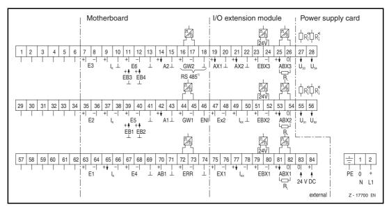
Fig. 19-5 Connection diagram of field case / Control panel case
