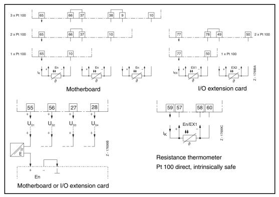
Fig. 19-6 Terminal assignment (field case/control panel case) for resistance thermometer Pt 100 direct and for two-wire transmitter
