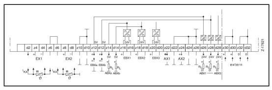
Fig. 19-2 Connection diagram of 19" plug-in card - I/O extension card
