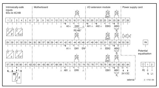
Fig. 19-7 Connection diagram of field case with intrinsically safe inputs (see "Expert Commentary" No. 95-04-205-Ex)
