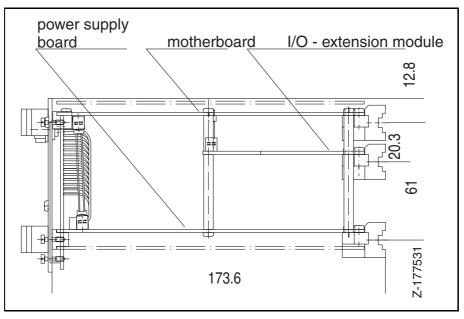
Fig. 16-2 Dimensional drawing of 19" plug-in card (dimensions in mm)
