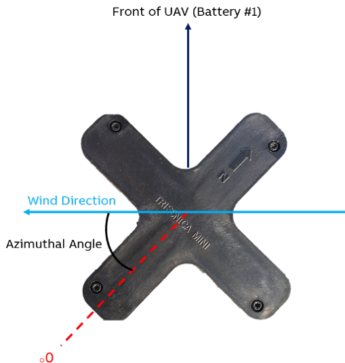
Figure 145 Azimuth Angle Definition for a Given Wind Direction
