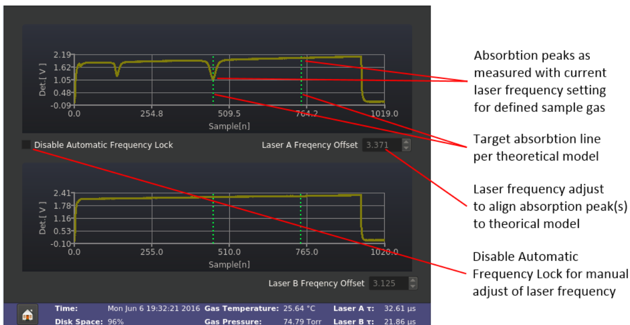
Figure 33: Laser Adjust for Optimizing Measurement Calibration
