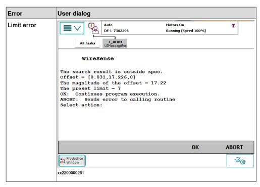
When the above shown dialog is active, the signal  $ws\_do\_Dialog\_X$  will be high and  $ws\_go\_Dialog\_X$  will be set to 14. The remote device may respond to the dialog by setting  $ws\_gi\_Response\_X$  to a value from the list below, followed by pulsing  $wi\_di\_Ack\_X$ .
