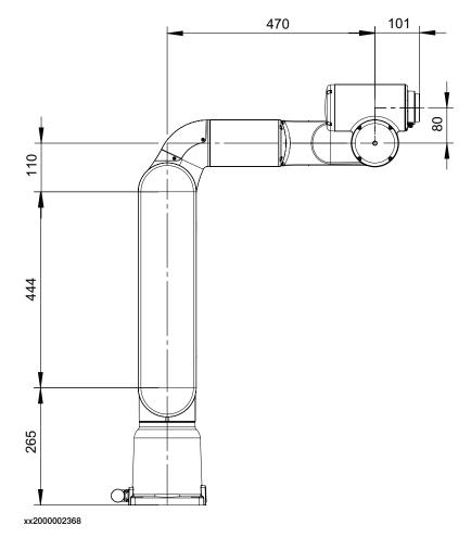
1.3.4 Fitting equipment on the robot (robot dimensions) *Continued*
