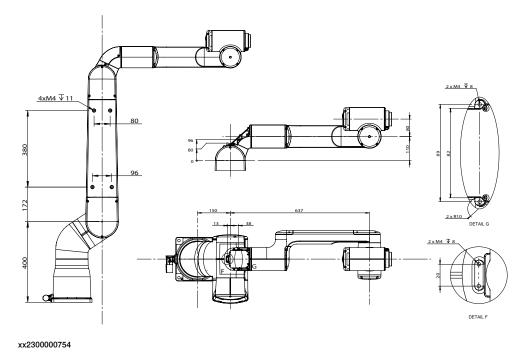
1.3.4 Fitting equipment on the robot (robot dimensions) *Continued*
