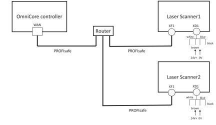
2 PROFIsafe-based laser scanners (option 3051-3), without PLC connected
