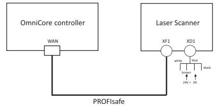
1 PROFIsafe-based laser scanner (option 3051-1), without PLC connected
