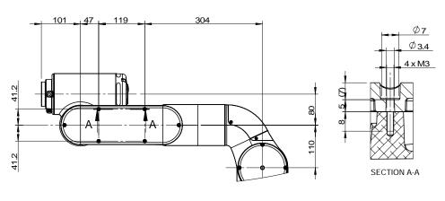
3.3.8 Fitting equipment on the robot (robot dimensions) *Continued*
