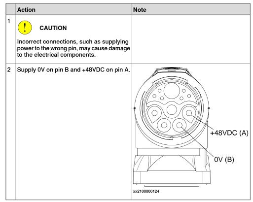
3.3.5 Installation of brake release tool
