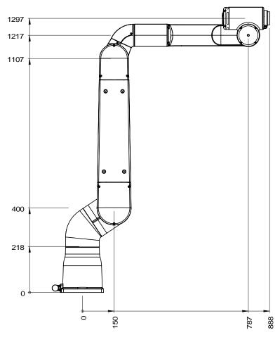
3.3.8 Fitting equipment on the robot (robot dimensions) *Continued*
