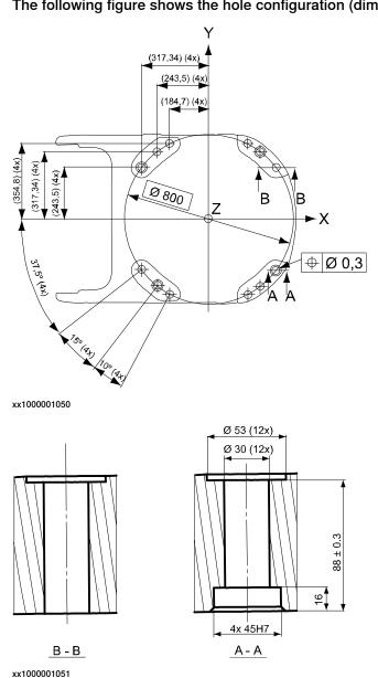
Fastening holes robot base The following figure shows the hole configuration (dimensions in mm).
