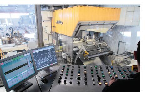
Profilglass SpA's four cold rolling mills plus the tension leveling line are running with 4 Stressometer systems, 6 MTG-gauges, 3 Strip Scanner systems and 8 tension load cells.
