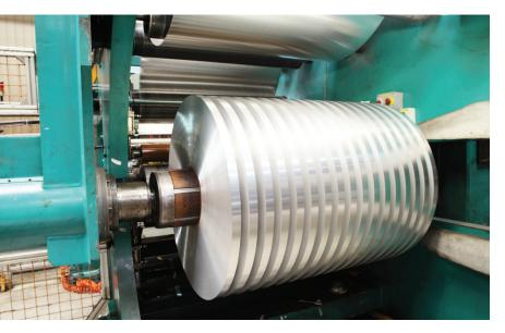
Gränges Shanghai's (former Sapa Shanghai) rolling mills and process lines are running with 6 Stressometer systems, 7 MTG-gauges, 2 Strip Scanner systems and around 30 tension load cells.
