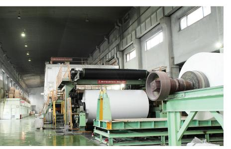
Shanghai Prosperous Paper's winders and calenders are running with Pressductor PillowBlock load cells providing an accurate web tension measurement.
