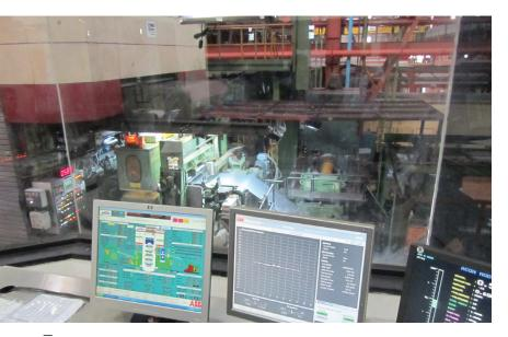
JSW Steel's 2-stand compact cold rolling mill and skinpass mill running with two Stressometer 7.0 FSA flatness control systems.
