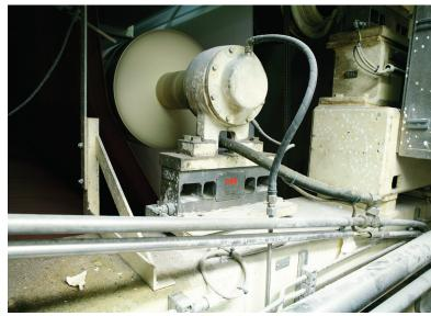
01 In the dryer section with high humidity and temperatures up to 90°C it is very important with ABB's reliable tension measurement.
