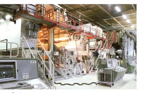
Stora Enso Fors' machines for manufacturing of carton board are running with Pressductor PillowBlock load cells providing accurate wire and web tension measurement.
