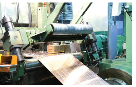
Aurubis Finland's (former Luvata Copper) three rolling mills are running with three double systems with all together six MTG thickness gauges.
