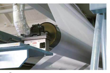
Ahlstrom-Munksjö Paper Billingsfors' paper machines and winders are running with Pressductor PillowBlock load cells and Pressductor Radial Tensiometers (PRT load cells) providing an accurate web tension measurement.
