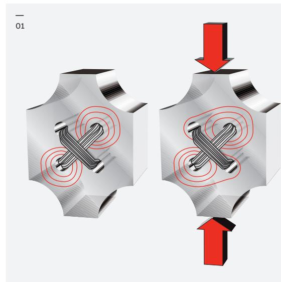
Mechanically, the load cell is virtually a solid block of stainless steel. Its consequent overall strength and rigidity with a high spring constant are important contributions to applications that put a premium on overload protection or are sensitive to vibrations.
