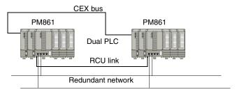
Figure 5. Example of a redundant CPU configuration.
