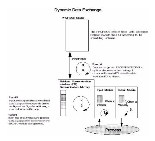
Figure 8. Transportation of dynamic data between PROFIBUS-DP/DPV1 master and S800 I/O modules.
