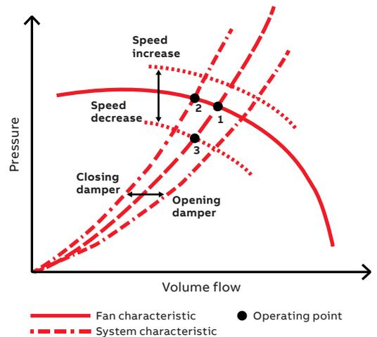
Fig. 2: Typical fan characteristic showing operating point
