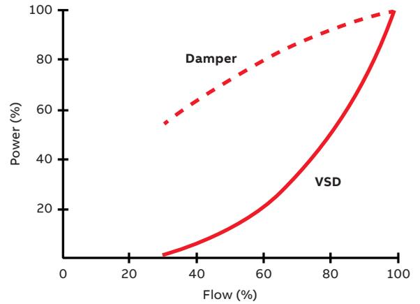
Fig. 1: Graph showing fan power requirements for damper and variable speed drive (VSD)
