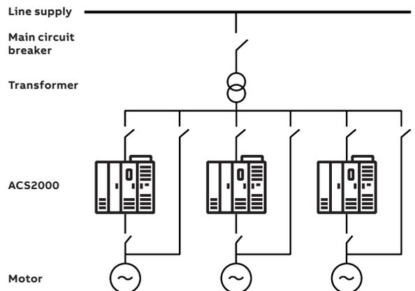
Fig. 3: The three ACS2000 direct-to-line variable speed drives are connected to the same network, requiring only one transformer.
