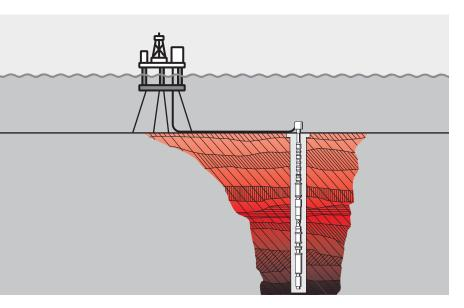
Electrical Submersible Pumps (ESPs) provide artificial lift in oil wells where there is insufficient natural flow.
