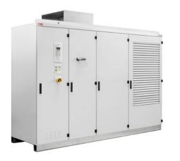
ABB's ACS1000i 3.3 kV medium voltage drive uses a drive cubicle in which transformer, contactor and on-board auxiliary power supply are built-in. operation. By having a matched system, the motor and the variable speed drives from the same supplier, ensures that optimum performance of the products is achieved.
