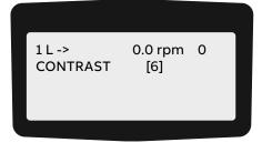
5. To confirm the selection and to return to the actual signals display, press the ENTER key.
