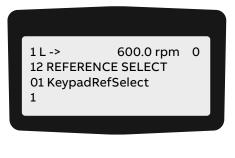
2. To select a different group, press the corresponding fast navigation key.
