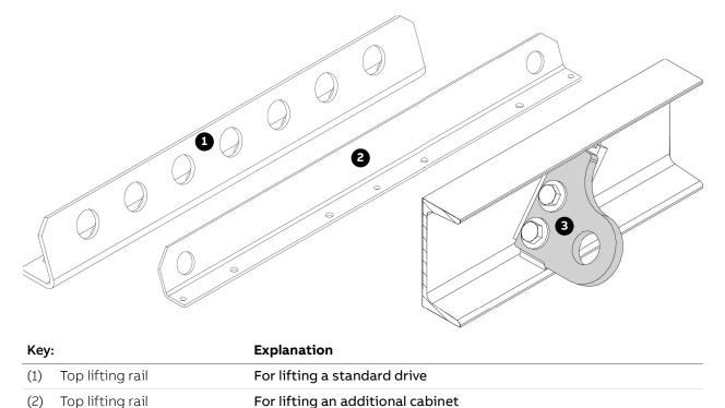
On base frame for lifting the drive
