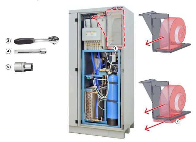
Fig. 80. Water cooling unit – replacing the internal fan
