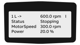
NOTE – As long as the stop sequence is in progress, the drive can always be restarted by pressing the **START** key on the CDP control panel.
