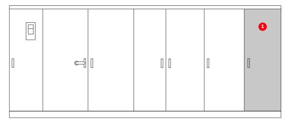
Fig. 16. ACS1000W water-cooled with (1) braking chopper
