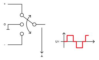
Fig. 15. Three-level voltage source inverter principle
