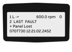
4. To clear the fault memory, press the RESET key.
