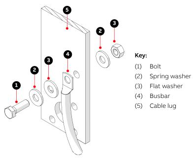
Fig. 59. Bolted busbar connections
