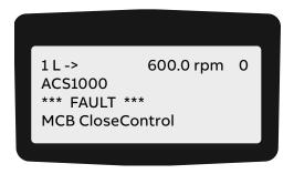
The message can be saved and viewed in the fault history of the drive when a PC with the DriveWindow or DriveDebug is connected to the drive. The fault logger can also be called up on the CDP control panel.
