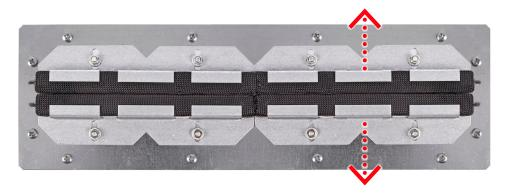
5. If the outer cable screen is non-conductive, cut open the cable screen in the middle of the stripped area (1), pull the screen ends over the cable insulation (2) and then connect the screen ends with a continuous conducting foil (3).
