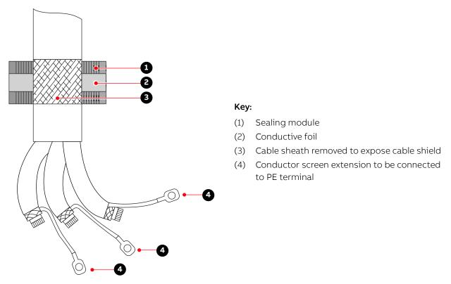
Fig. 63. Preparing control cables for sealing modules
