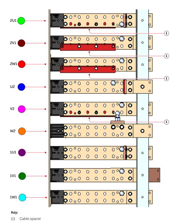
Fig. 52. Example of busbars with cable spacers - cable entry top
