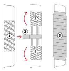
Fig. 61. Preparing control cables for EMC plates
