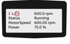
NOTE – If you change the direction while the motor is running, the motor automatically ramps down to zero speed and re-accelerates in the opposite direction to the preset speed. The arrow changes at zero speed.
