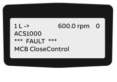
2. To reset the fault, press the **RESET** key.
