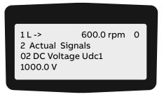
5. To confirm the selection and to return to the actual signals mode, press the **Enter** key.
