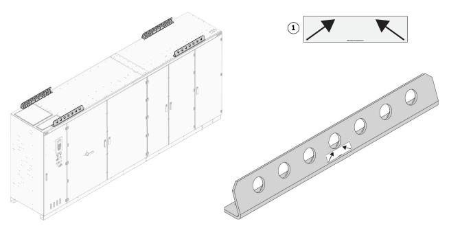
Fig. 34. Top lifting rails with recommended lifting points
