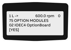
6. To confirm the selection and to return to the actual signals display, press the ENTER key.
