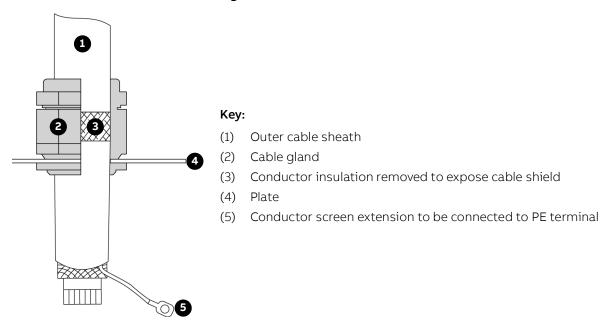
Fig. 64. Preparing control cables for cable glands
