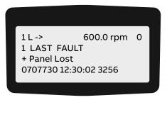
3. To display a specific fault, press the slow navigation keys.
