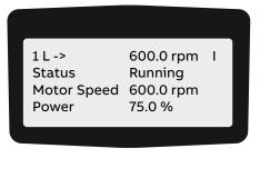
To select a line where the actual signal is to be displayed, press the corresponding slow navigation key.
