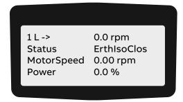
2. To de-energize the drive completely, switch off and lockout all auxiliary voltages from external sources.
