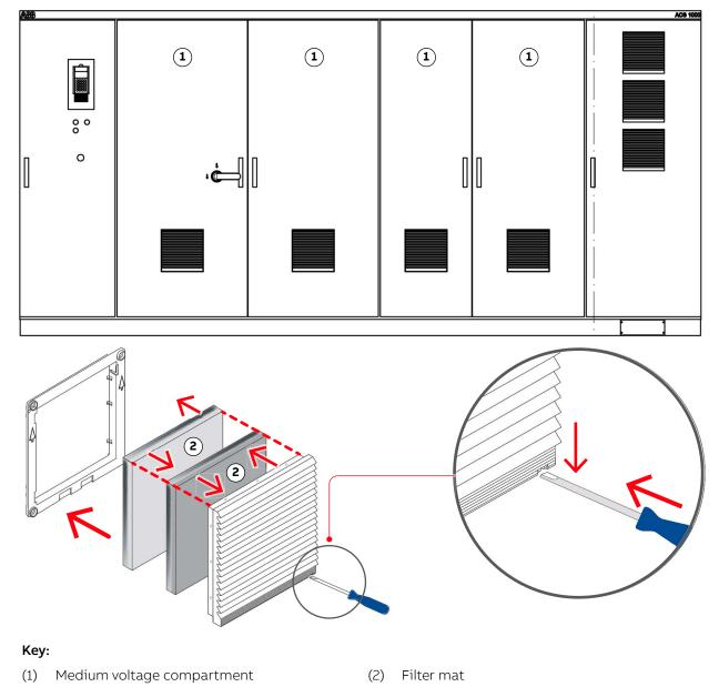
Fig. 76. Cleaning and replacing filter mats
