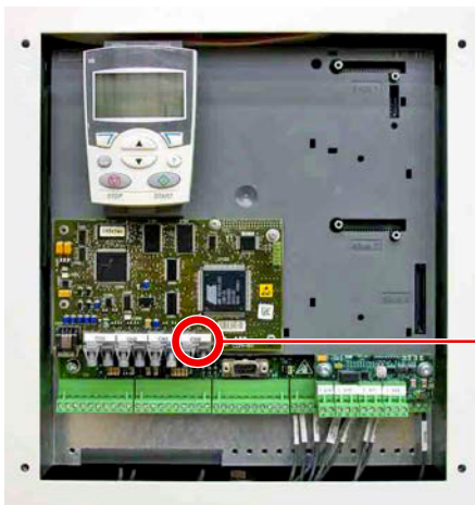
Figure 6-40 COM-8x circuit board (A) in a DCS800 converter (ED7Y type) and a detail of channel CH0 (B) on the board
