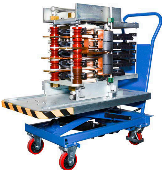
Figure 6–1 Phase module on lift table
