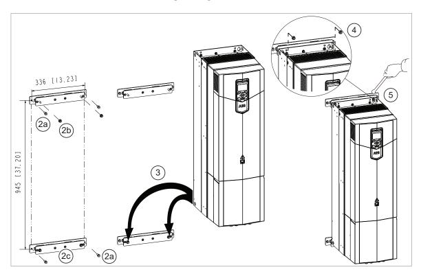
2 Vibration dampers (option +C131) for ACS880-11 and ACS880-31 frame R8 drives installation instructions
