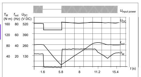
$U_{\rm DC}$  = Intermediate circuit voltage of the drive,  $f_{\rm out}$  = Output frequency of the drive,  $T_{\rm M}$  = Motor torque
