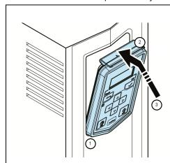
To attach the control panel to a drive:
