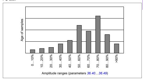
Amplitude logger 1 is fixed to monitor motor current, and cannot be reset. With amplitude logger 1, 100% corresponds to the maximum output current of the drive  $(I_{\text{max}})$ , which is listed in the *Hardware manual* of the drive. The measured current is logged continuously. The distribution of samples is shown by parameters 36.20...36.29.
