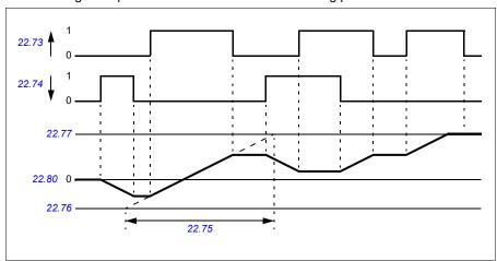
Parameters 22.73 Motor potentiometer up source and 22.74 Motor potentiometer down source control speed or frequency from zero to maximum speed or frequency. The running direction can be changed with parameter 20.04 Ext1 in2 source. See the following example.
