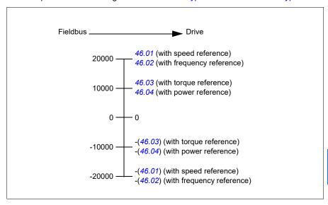
The scaled references are shown by parameters 03.09 EFB reference 1 and 03.10 EFB reference 2.
