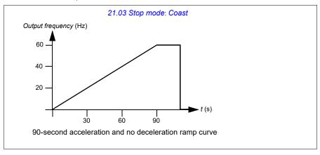
In pump applications, the stop mode is typically set to ramp and the deceleration ramp is used while stopping. Ramping a pump motor to a stop helps prevent issues
