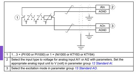
WARNING! As the inputs pictured above are not insulated according to IEC 60664, the connection of the motor temperature sensor requires double or reinforced insulation between motor live parts and the sensor. If the assembly does not fulfill the requirement, the I/O board terminals must be protected against contact and must not be connected to other equipment or the temperature sensor must be isolated from the I/O terminals.
