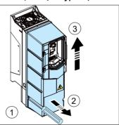
7. Frames R1...R2 and R6...R9, IP21 (UL Type 1): Install the cable/conduit box
