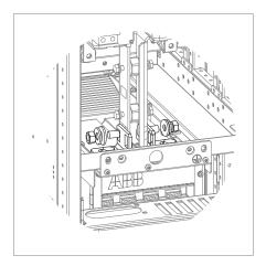
7. Close the inlet valve (a) and outlet valve (located on the right-hand side of the cubicle). Lead the drain hoses (b, on both sides of the cubicle) into a suitable container. Open the drain valves (c, on both sides of the cubicle). This will drain all modules in the cubicle.
