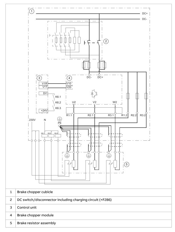
This diagram shows the brake resistor cable connections and an example connection of the thermal switches.
