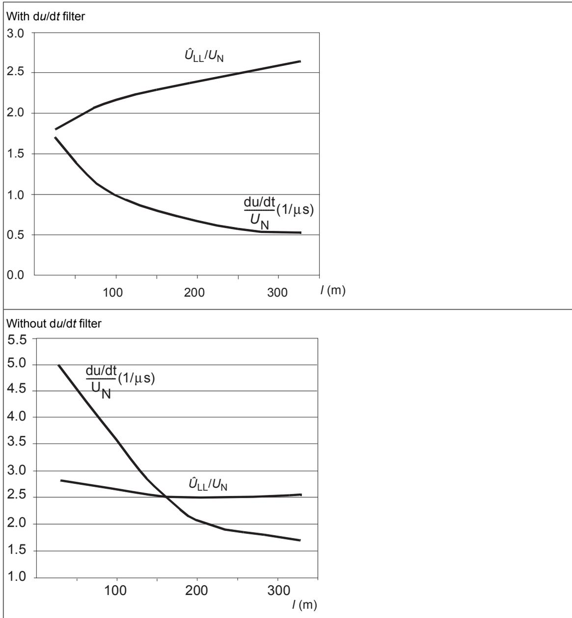
ACS580-07, ACH580-07 and ACQ580-07: A with du/dt filter, B without du/dt filter
