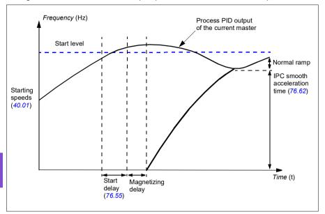
The figure below shows the smooth pump transitions with different ramp times.
