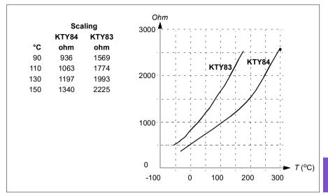
The figure and table below show typical KTY83 sensor resistance values as a function of the motor operating temperature.
