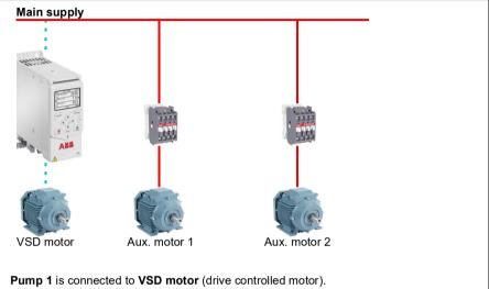
Pump 1 is connected to VSD motor (drive controlled motor) Pump 2 is connected to auxiliary motor 1. Pump 3 is connected to auxiliary motor 2.
