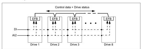
inverter-to-inverter link. These signals must be externally sent to each drive to ensure a redundant system.
