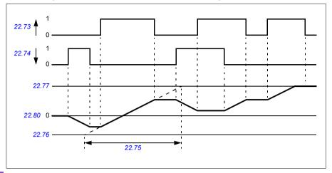
The following example shows the behavior of the Floating point control counter value.
