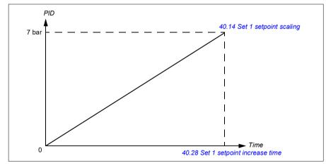
The figure below illustrates the operation of the Soft pipe fill function.
