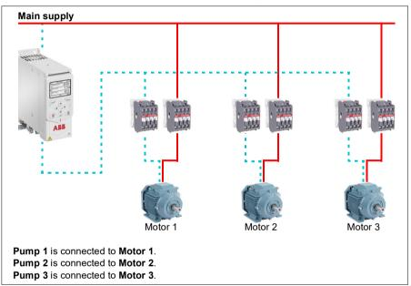
Example: Three-pump constant pressure water supply application
