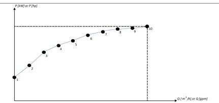
The flow calculated based on HQ or PQ curve is scaled according to the actual speed of the pump. Scaling reference speed is set in parameter *80.21 Flow pump nominal speed*.
