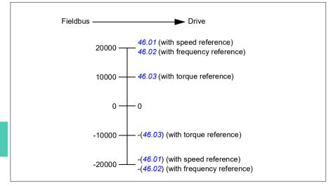
The scaled references are shown by parameters 03.05 FB A reference 1 and 03.06 FB A reference 2.
