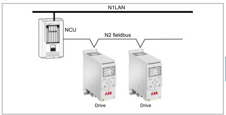
The following diagram shows the drive's integration to the Johnson Controls Metasys Companion system.
