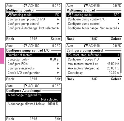
Multipump (IPC, intelligent pump control) systems allows up to 8 drives to be connected to each other. This menu contains programming assistants for load sharing, balancing the run time between the pumps and keeping each pump running optimally.
