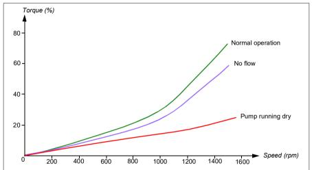
The figure below illustrates the operation of dry pump protection function.
