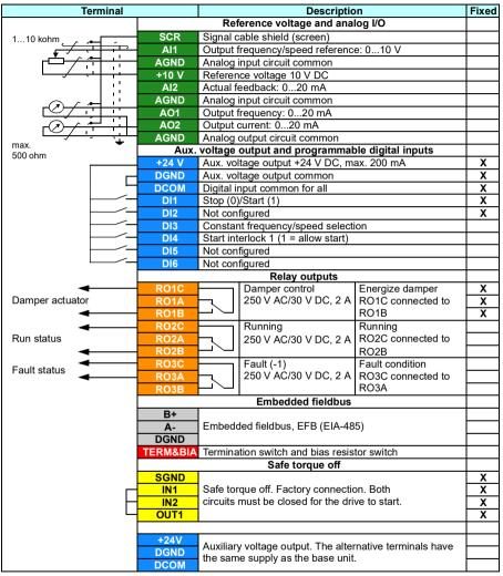
Terminal sizes: 0.14...1.5 mm<sup>2</sup> (26...16 AWG) Tightening torques: 0.5...0.6 N·m (4.4...5.3 lbf·in)
