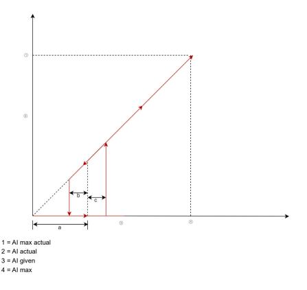
In the above diagram, a is the deadband value. Values b and c are -10% and +10% hysteresis value respectively. Hysteresis values are internally set in firmware and cannot be edited by the user.
