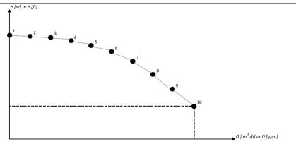
The figure below shows the PQ performance curve of the pump for the flow calculation function.
