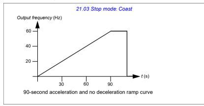
In pump applications, the stop mode is typically set to ramp and the deceleration ramp is used while stopping. Ramping a pump motor to a stop helps prevent issues
