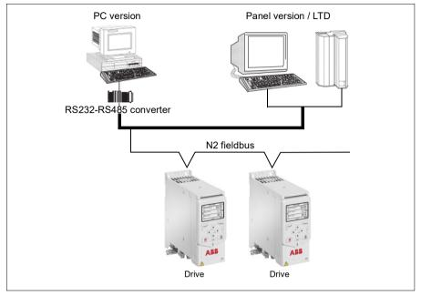
On the N2 fieldbus each drive can be accessed by the full complement of Metasys FMS features, including change-of-state (COS) monitoring, alarm notification, scheduling, trend, and totalization.
