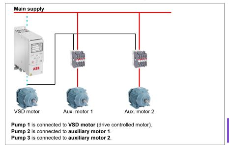
**Example:** Three-pump constant pressure water supply application
