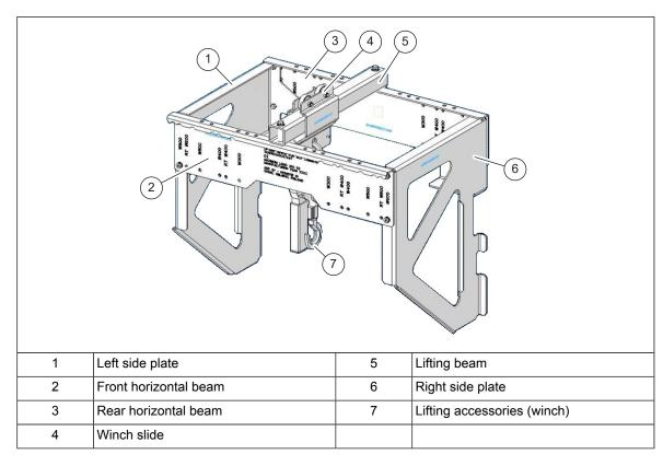
The figures below shows the differences between the lifting device variants: The side support plates differ, otherwise the lifting devices are similar.
