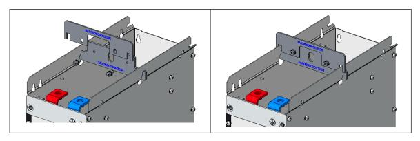
Install the lifting beam 3AXD50000195305 according to the illustration below. Use the two M12x25 bolts and M12 nuts in the package.
