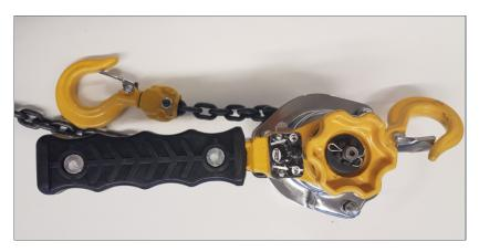
When using the winch, always make sure that the lifting hooks are locked before lifting or lowering. The winch has a lever with three positions: FREE, DOWN and UP. When using FREE position, the winch must be unloaded.
