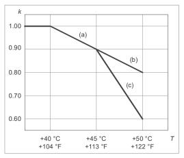
1-phase (NBRW-669) brake modules (option +D150): 0...50 °C (32...122 °F): no current derating required
