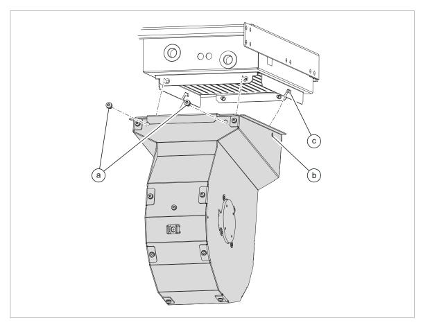
Replacing the common motor terminal cubicle fan
