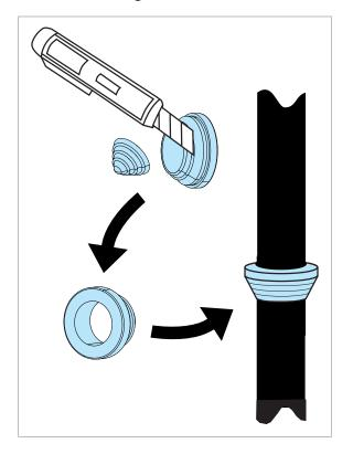
12. Attach the conductive sleeves to the cable shields with cable ties. Tie up the unused conductive sleeves with cable ties.
