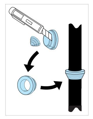
7. Attach the conductive sleeves to the cable shields with cable ties. Tie up the unused conductive sleeves with cable ties.
