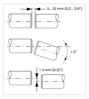
5. Center the Axilock connectors onto the gaps between coolant pipe ends. Tighten the connector screws to the torque indicated on the connector label.
