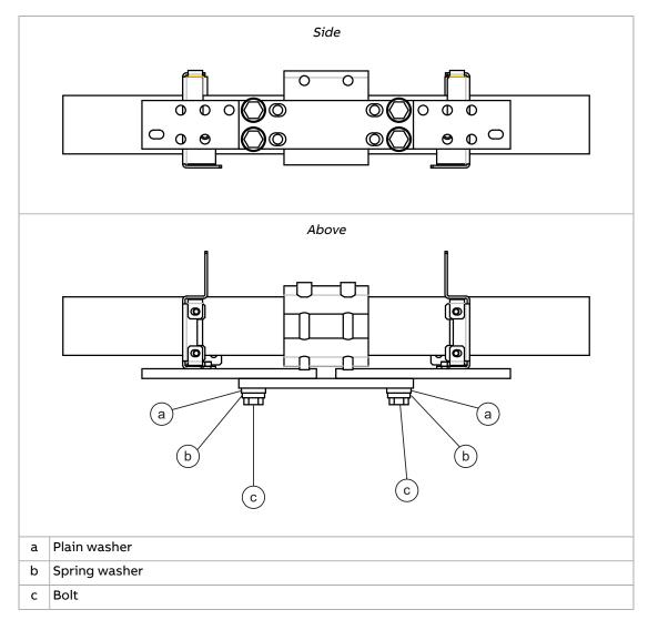
8. Connect the PE (ground) busbars using the M10 bolts included. Tighten to 35...40 N·m (25...30 lbf·ft).
