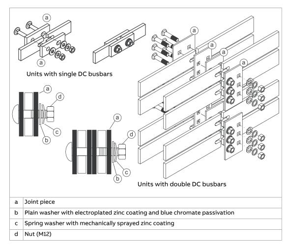
10. Connect the DC and AC busbars. Tighten the bolts to 55...70 N·m (40...50 lbf·ft).
