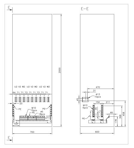
Inverter module cubicle with three R8i modules, bottom cable exit
