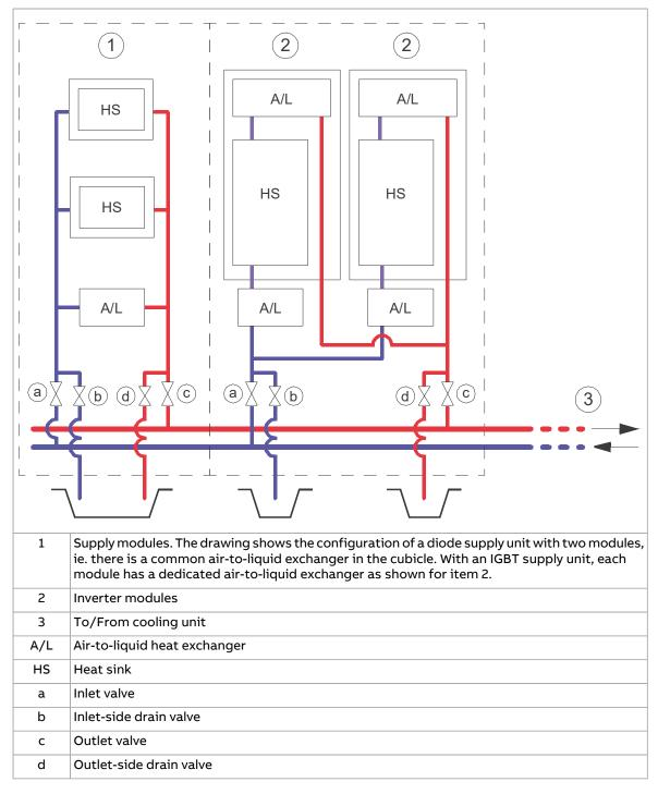
The coolant used with ACS880 liquid-cooled drive systems is Antifrogen<sup>®</sup> L 25% or 50% mixture. See Coolant specification (page 176).
