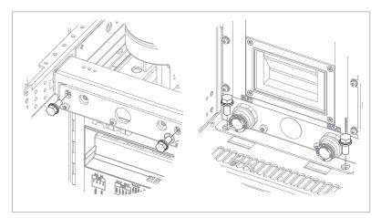
10. Pull the module carefully out onto the service platform. Keep the module secured to a hoist or equivalent to prevent the module from falling. For information on using the lifting device, see Converter module lifting device for drive cabinets hardware manual (3AXD50000210268 [English]).
