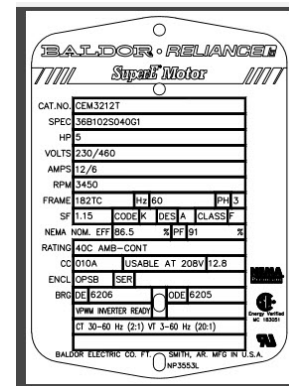
Example of a nameplate of an induction (asynchronous) motor.
