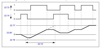
Parameters 22.73 Motor potentiometer up source and 22.74 Motor potentiometer down source control speed or frequency from zero to maximum speed or frequency. The running direction can be changed with parameter 20.04 Ext1 in2 source. See the following example.
