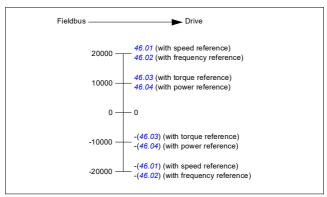
The scaled references are shown by parameters 03.09 EFB reference 1 and 03.10 FFB reference 2
