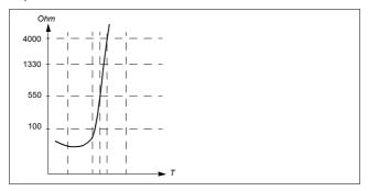
When an analog output is not available or used for other purposes, it is possible to setup a voltage divider connection that uses the internal resistance of a digital input. 1...3 PTC sensors can be connected in series with 10 V reference and digital and analog inputs. The temperature measurement function reads the voltage over the internal resistance of the digital input from the analog input and calculates the PTC resistance
