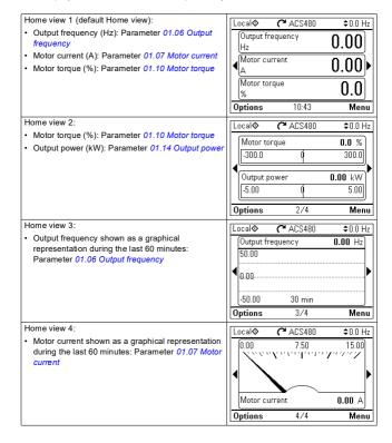
You can replace parameters in the Home view displays with other parameters or create new Home view displays showing selected parameters.
