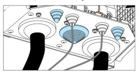
$\underline{\text{IP66 (UL Type 4X)}}$ : Plug unused holes with a hole plug with IP66 (UL Type 4X) or better protection rating and tighten securely.
