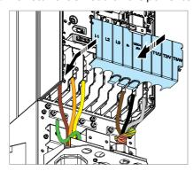
16. Secure the conduits outside the unit mechanically.
