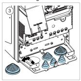
Note: The drive is shipped with grommet cones pointing up. They must be
