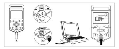
**Note:** For IP66 (UL Type 4X) drive, the USB connection on the panel cannot be accessed while the cover is in place. Use the Bluetooth functionality to troubleshoot the drive using the DriveTune app from your phone.
