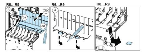
6. Remove the rubber grommets, if present, for the motor and input power cabling.
