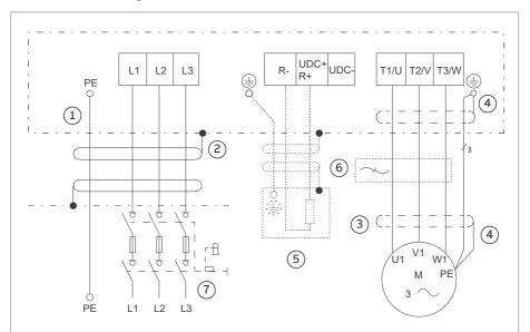
**Note:** UL (NEC) installation can include separate insulated conductors inside a conduit, shielded VFD cable in conduit, or shielded VFD cable without conduit. The normal dashed symbol (3) in this diagram represents the shield of shielded VFD cable. The same solid symbol (2) represents conduit.
