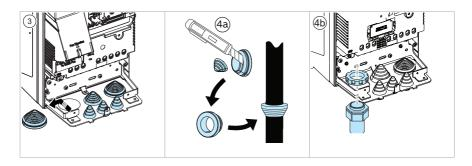
**Note:** If the drive is shipped with grommet cones pointing up they must be removed and inserted back pointing down.
