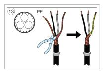
14. Connect the cable as the motor cable in step 7. Ground the shield 360 degrees (14a). Connect the twisted shield to the grounding terminal (14b) and the conductors to the R+ and R- terminals (14c) and tighten to the torque given in the table.
