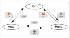
**Note:** When you restart the drive while fault 7081 Control panel loss is active, the mode changes from Hand or Off to Auto.
