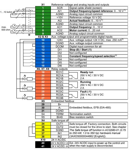
Total load capacity of the Auxiliary voltage output +24V (X2:10) is 6.0 W (250 mA / 24 V DC).
