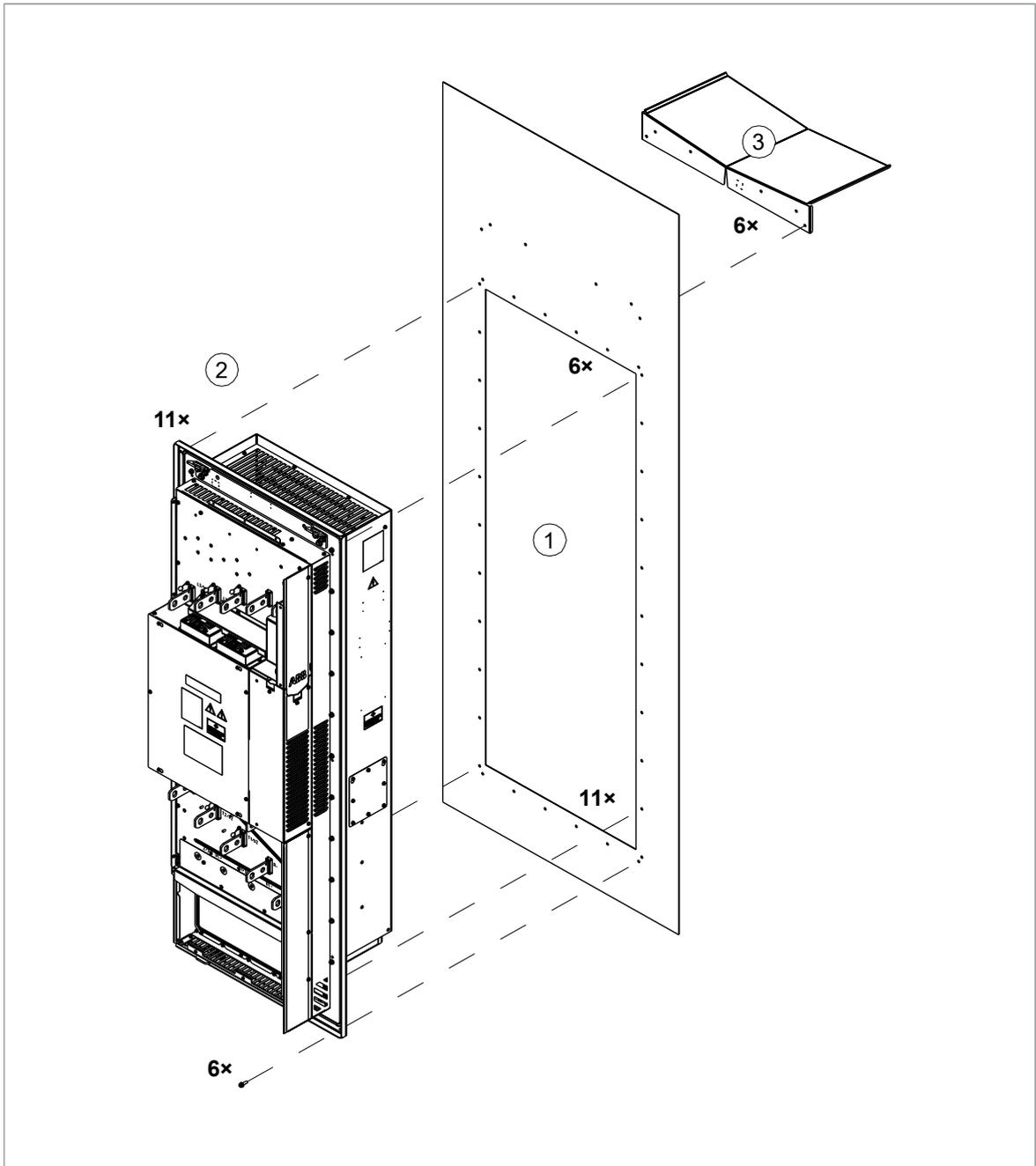
■ **Attaching the drive module by the heatsink**
