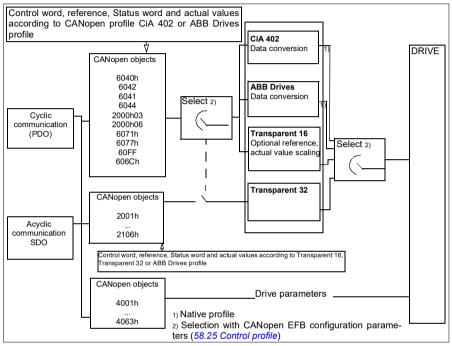
CANopen embedded fieldbus interface operation
