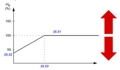
The red arrows indicate the drive output frequency. Higher value increases the motor overload level, and lower value decreases it.
