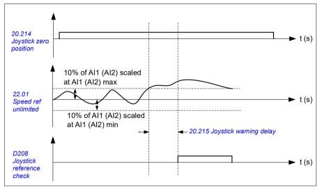
The diagram shows the operation of the *Joystick reference check* warning.
