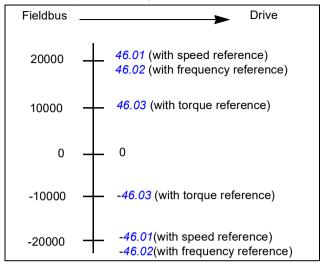
ABB Drives profile scaling from drive to fieldbus
