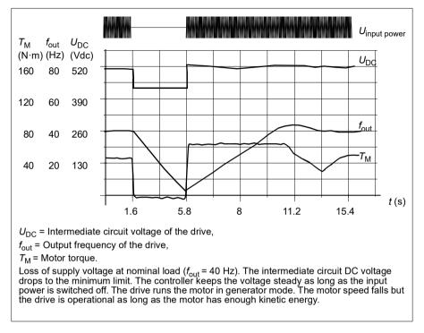
**Note:** Units equipped with a main contactor must be equipped with a hold circuit (e.g. UPS) to keep the contactor control circuit closed during a short supply break.
