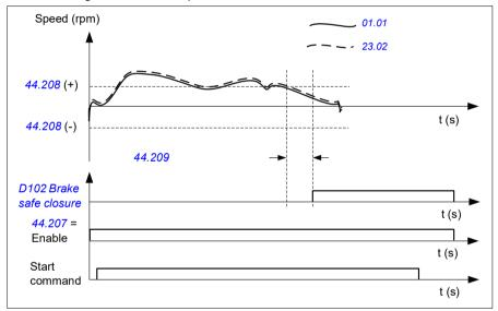
The below diagram shows the operation of the Brake safe closure fault.
