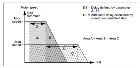
Speed compensation does not take into account shape times (23.32 Shape time 1 and 23.33 Shape time 2). Positive shape times lengthen the distance traveled.
