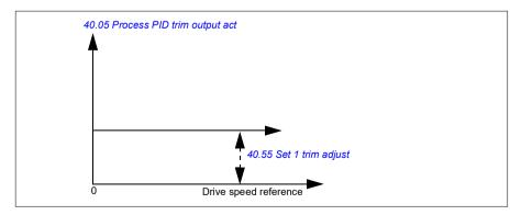
**Note:** In the above graph, it is assumed that the PID output is limited or stable at 100. This is for clarity only. In real life scenarios, the PID output can vary based on the setpoint and the actual value.
