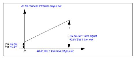
**Note:** In the above graph, it is assumed that the PID output is limited or stable at 100. This is for clarity only. In real life scenarios, PID output can vary based on the setpoint and actual.
