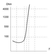
When analog output is not available or used for other purposes, it is possible to set up a voltage divider utilizing internal resistance of a digital input. 1...3 PTC sensors are connected in series to 10V reference and Digital and Analog inputs. The voltage over the digital input internal resistance varies depending on the PTC resistance. The temperature measurement function reads the voltage over the sensor from the analog input and calculates the resistance.
