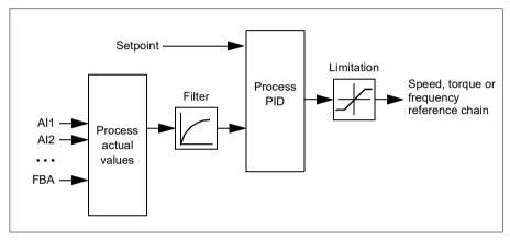
The simplified block diagram below illustrates the process PID control.
