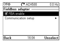
Use the settings in the Fieldbus adapter submenu to use the drive with the following fieldbus protocols, shown with the optional fieldbus adapter module required:
