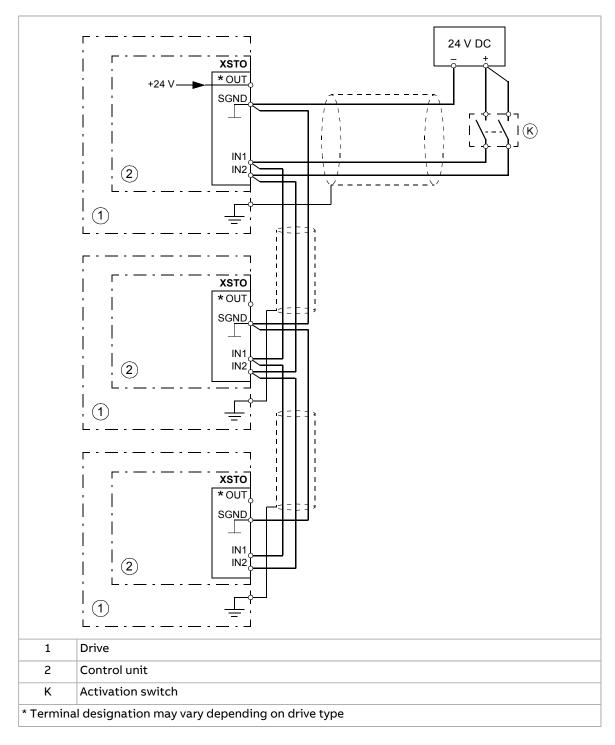
External power supply (example, drives with ZCU-xx and BCU-x2)
