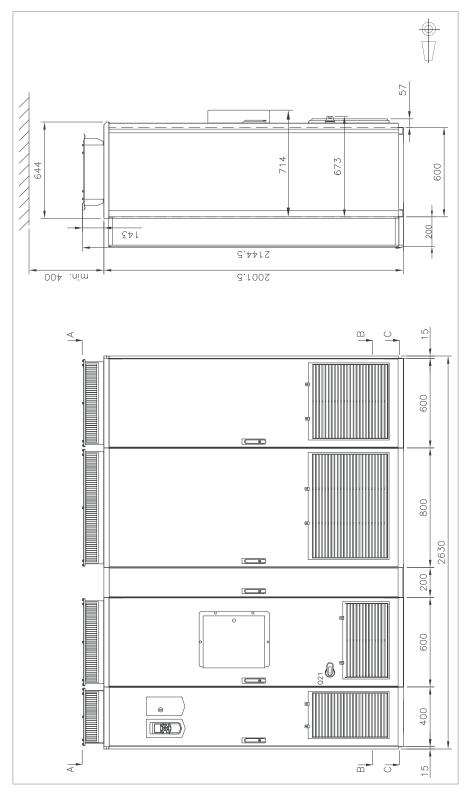
Frame 2×R8i+2×R8i with main breaker (+F255) and common motor terminal cubicle (+H359), 1/2
