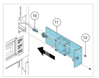
Replacing the cooling fan in the auxiliary control cubicle
