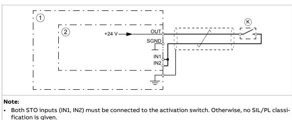
• Pay special attention to avoiding any potential failure modes for the wiring. For example, use shielded cable. For measures for fault exclusion of wiring, see eg. EN ISO 13849-2:2012, table D.4.
