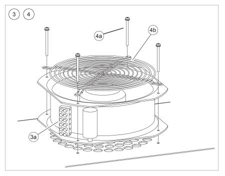
Replacing a roof fan (IP54/UL type 12)
