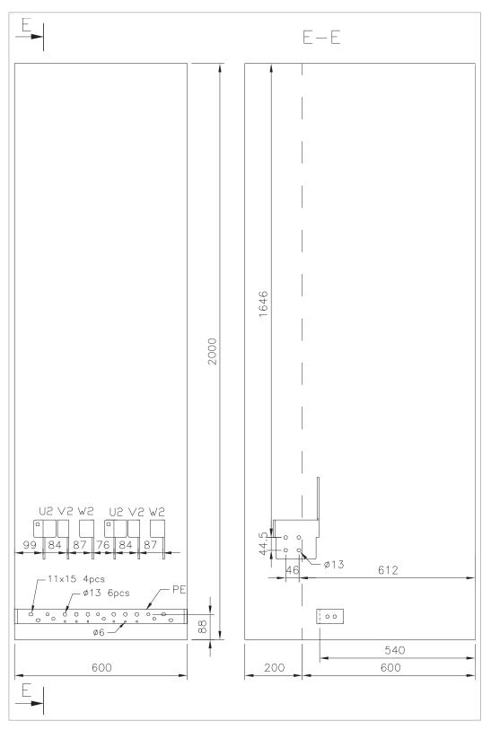
Inverter module cubicle with two R8i modules, top cable exit
