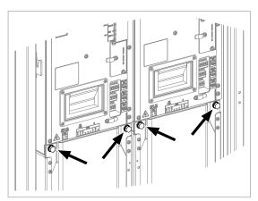
b. Reinstall the transverse retaining bracket. At the ends of the bracket, tighten the screws to 9 N·m [6.6 lbf·ft]. Reinstall the fan carriage bolts removed at previous step, and tighten to 22 N·m (16 lbf·ft).
