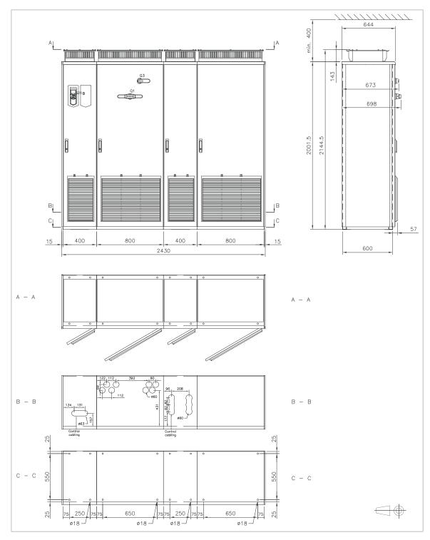
Frame 1×R8i+1×R8i with brake choppers and resistors (+D150+D151)
