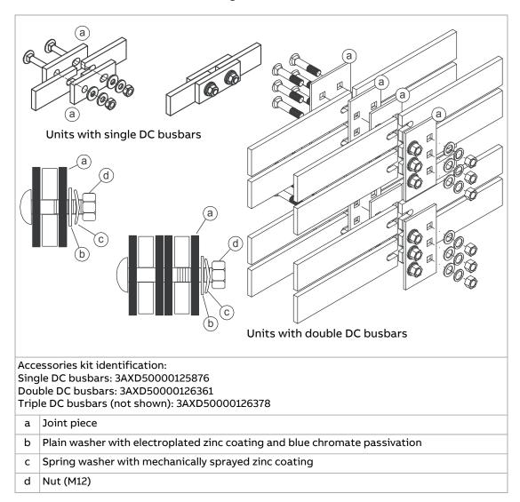
8. Connect the DC and AC busbars. Tighten the bolts to 55...70 N·m (40...50 lbf·ft).
