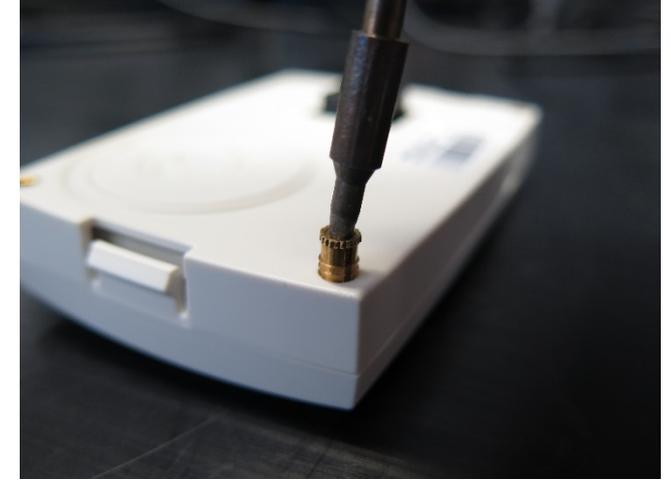
3. Heat the soldering iron to 350°C and heat the insert for two seconds.
