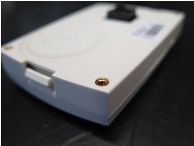
4. Push the insert into the hole with the hot soldering iron. Make sure the insert is in level with the panel's back cover
