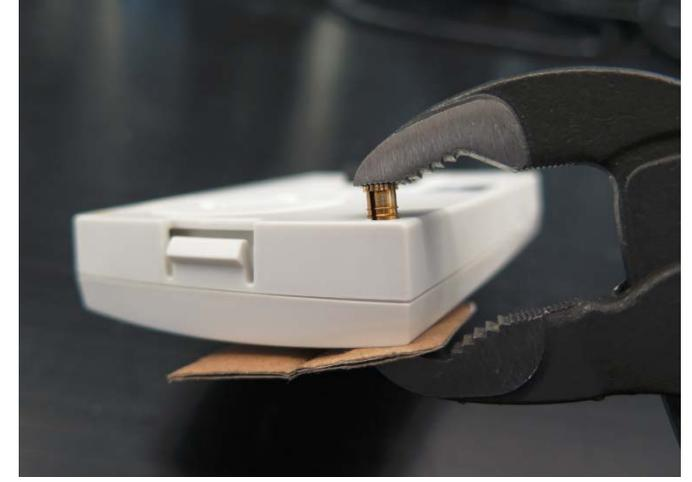
3. Cover the front of the panel and squeeze the insert into the panel with pliers.
