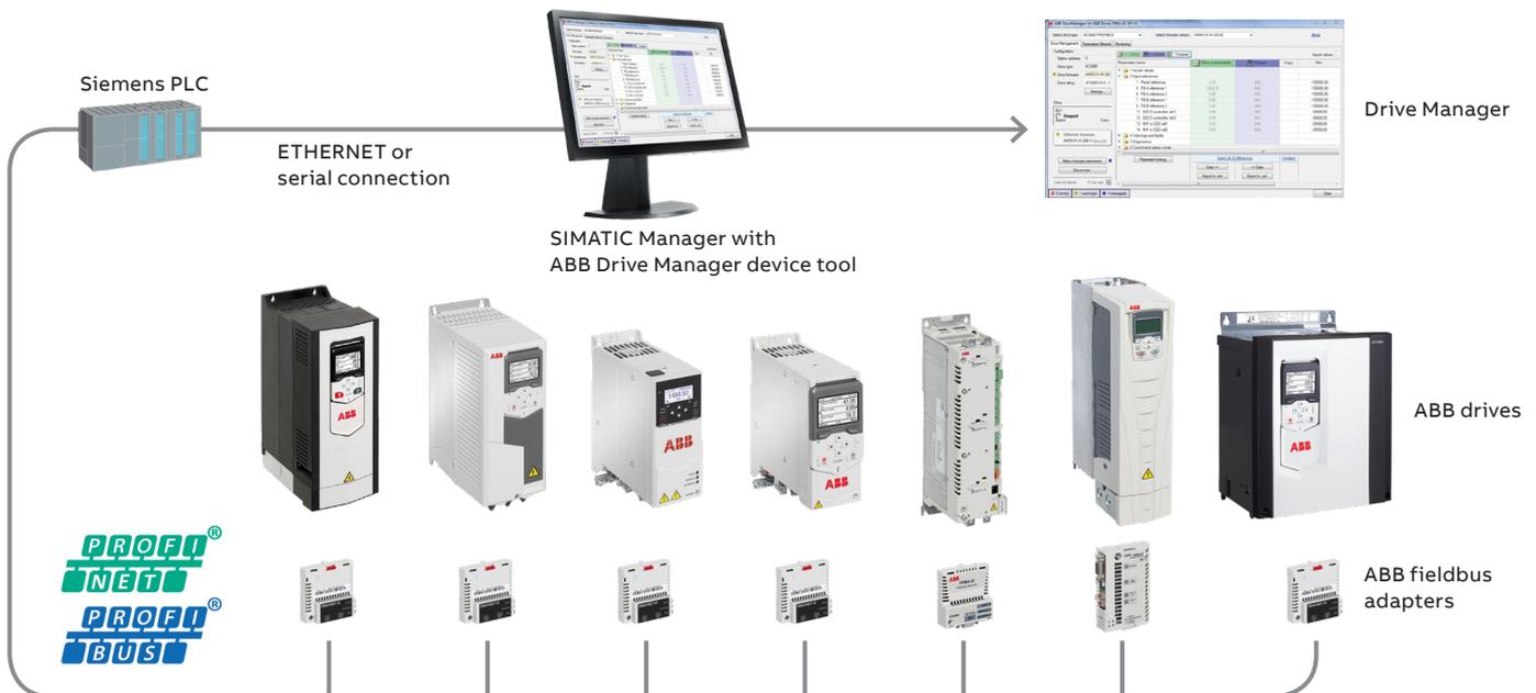
Drive Manager for SIMATIC is a plug-in device tool that can be easily installed into the STEP 7 and TIA Portal. It utilizes the TCI interface of the SIMATIC PLC to communicate with the drives connected to PROFIBUS or PROFINET network.
