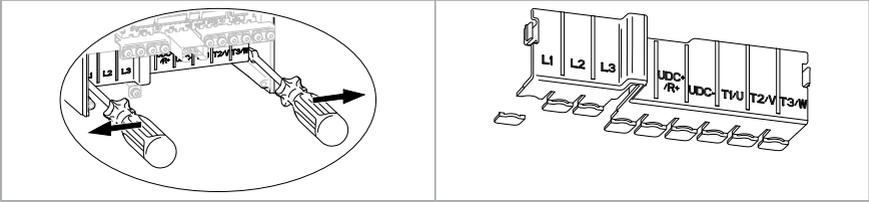
3. Attach the mechanical support shelf for the power cables to the drive module.
