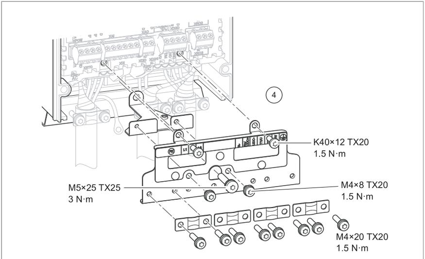
5. Connect the additional PE conductor of the input cable to the grounding shelf.
