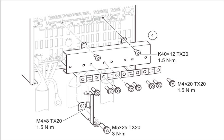
5. Connect the additional PE conductor of the input cable to the grounding shelf.
