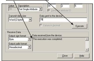
14. The power on the drive (RETA-01) will need to be turned off and back on, or a 51.27 (Parameter Refresh) to program the new Datawords in the RETA-01.
