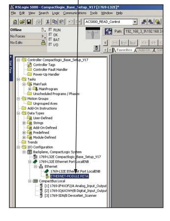
4. The Input and Output assembly size will need to be adjusted for the amount of Datawords for the RETA. The example within this instruction Dataword 5 In/Out has been enabled. The new Input word size is 5 and the Output word size is also 5.
