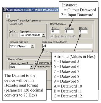
13. Click the Execute button to program the Dataword and the following message should be displayed in the Data received from device area below.
