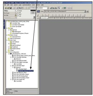
3. Click the Connection tab within the Module Properties window and then check the box to Inhibit Module
