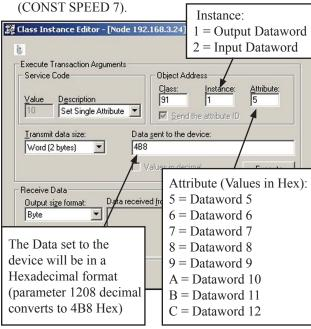
11. Click the Execute button to program the Dataword and the following message should be displayed in the Data received from the device area below.
