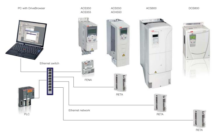
PC connected to drives using the same Ethernet network as the PLC.
