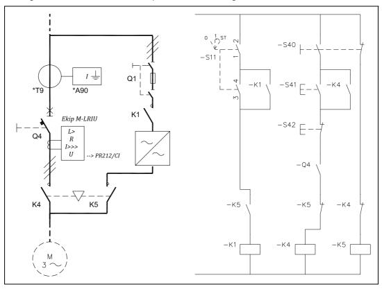
If the motor protection breaker Emax is used, the design is slightly different (implementation of K4 and Q4).
