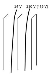
Lead 24 V and 230 V (115 V) control cables in separate ducts inside the cabinet.
