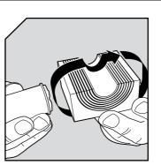
Lubricate all modules for the frame thoroughly on both the inside and the outside surfaces.
