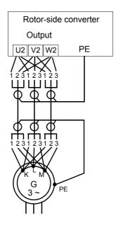
For information on how to change the rotation direction of the generator, see *ACS800-67LC system description and start-up guide* [3AUA0000059432 (English)].
