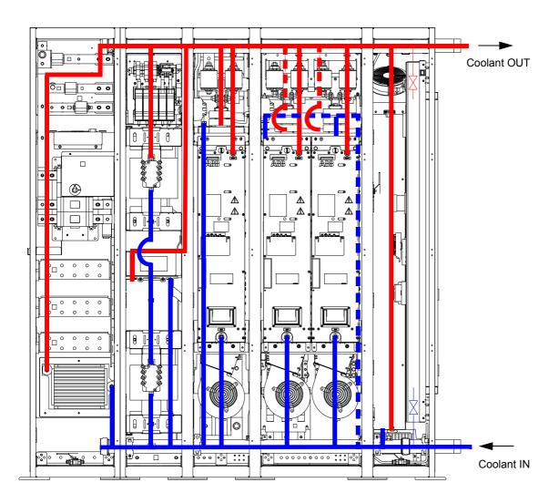
The power modules in each cubicle can not be isolated from the main cooling circuit. The converter is equipped with a drain valve and a bleed valve.
