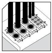
Mount the modules row by row starting from the inside. Precompress the frame.
