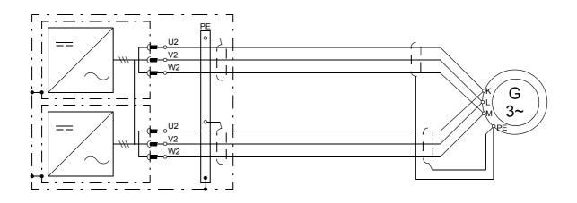
**Note:** Rotor-side cable connection terminals are U2, V2, W2 and PE. To be wired by the user. For selection of the cables, see chapter *Planning the electrical installation*. For the terminal sizes, tightening torques and lead-throughs, see chapter *Technical data*.
