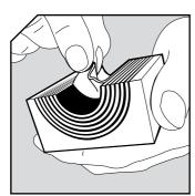
Adapt modules, which are to hold cables, by peeling off layers until you reach the gap seen in the next picture. Try to remove the same number of layers on both module halves.
