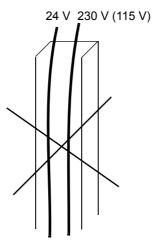
Not allowed unless the 24 V cable is insulated for 230 V (115 V) or insulated with an insulation sleeving for 230 V (115 V).
