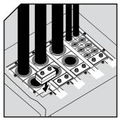
Lubricate the compression units. Insert one in the top of each opening.
