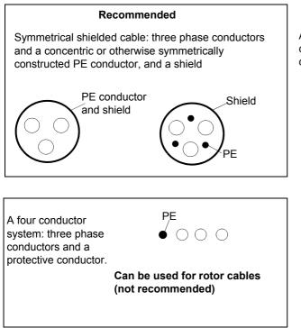
A separate PE conductor is required if the conductivity of the cable shield is <50% of the conductivity of the phase conductor.
