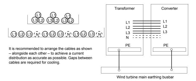
**Note:** Current derating of the cables is required when installing the cables in a cable tray. This derating factor must be taken into account as per the local electrical safety code.
