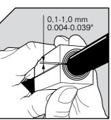
Achieve a 0.1...1.0 mm gap between the two halves when held against the cable.
